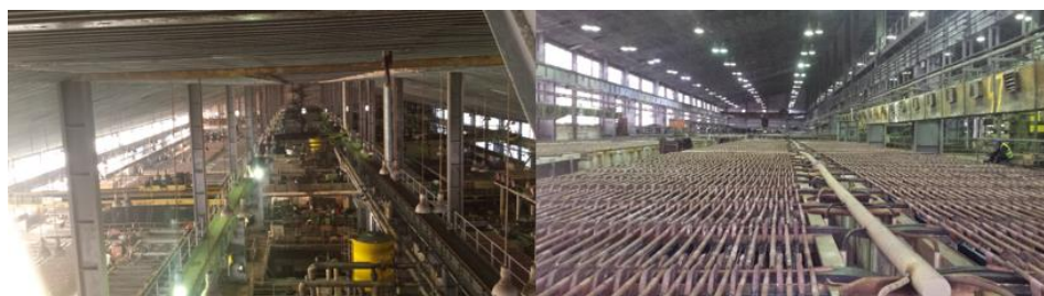
Figure 2 Interior of the electrolysis plant; view from the interior balcony where specimens were placed (left) and the ground floor with the pools where the electrolysis of copper anodes were carried out
