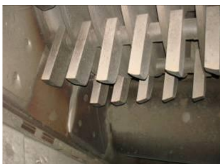
Figure 3 and Figure 4 Shaft with hammers and lower impact roller [1]
