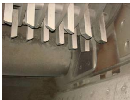
Figure 3 and Figure 4 Shaft with hammers and lower impact roller [1]
