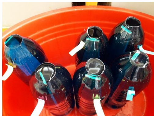
Figure 1 Continuous immersion testing of specimens
