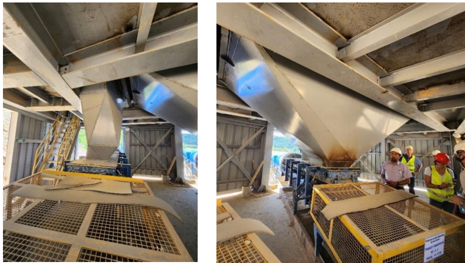
Figure 5 Storage of conveyors 4.3 and 4.4 with chutes with Flip-Flow sieves - finished state
