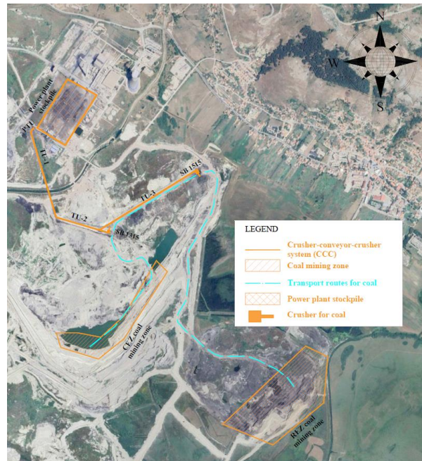
Figure 2 Spatial arrangement of zones where the coal exploitation is planned, network of transport roads and positions of facilities within the continuous part of coal transport system [14]
