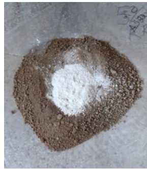
Figure 2 Homogenization material of subsoil with 5% lime
