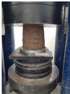
Figure 3 Uniaxial compressive strength of soil material
