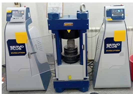
Figure 2 Device for compressive strength measurement
