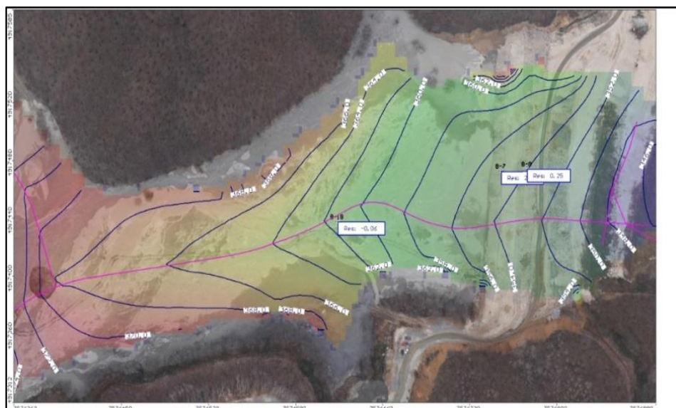
Figure 3 Map of hydroisohypsies and residual differences based on measurements from April 2024
