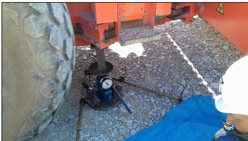
Figure 1 Performing a test using the static load plate
