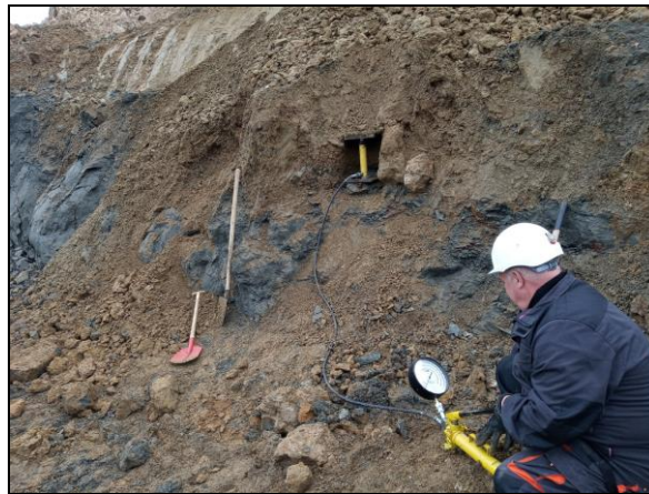
Figure 2.2 Appearance of a build-in shear equipment in the field
