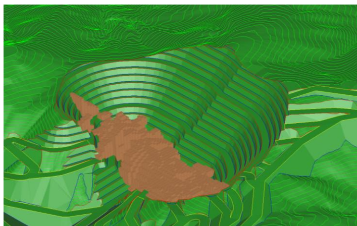
Figure 5 The appearance of the final contour of the open pit with a presentation of the block model for the Višnjica-Žuta Prla-Razvršje deposit (Gems software)
