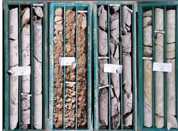
Figure 1 Marking core for geotechnical mapping
