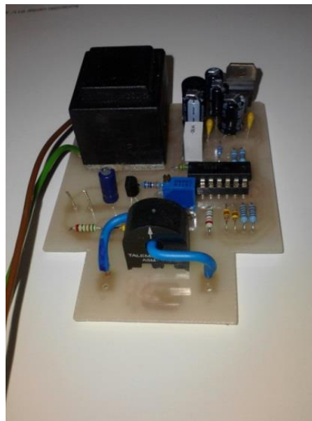
Figure 3 Single-sided transducer's PCB with the attached components
