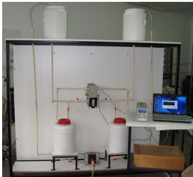
Figure 2 Pilot plant for the electrochemical synthesis of ferrate(VI)
