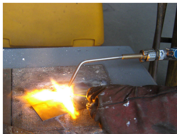
Fig. 2. Execution of the brazed overlap joint
