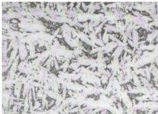
Figure 2 Microstructure of alloy, hot deformed (x960)
