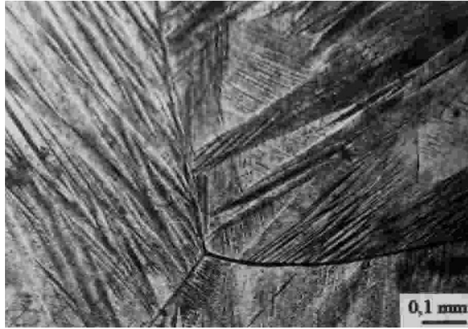
Fig. 4 Typical microstructure observed for the Cu-Zn-Al alloy The internal friction ( Q^{-1} ) as a function of temperature of the Cu-Zn-Al cantilever type sample is shown in Fig. 5.
