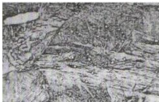
Figure 3 Microstructure of alloy, annealed at 850°C for 10 min and water quenched (x960)
