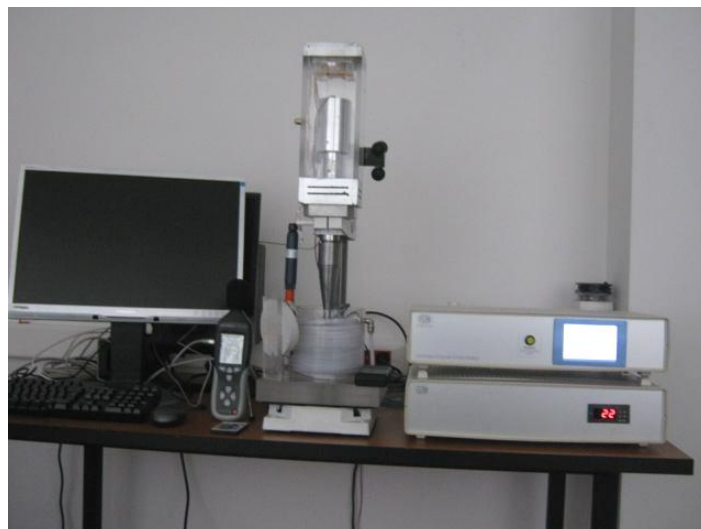
Fig. 1 Vibration apparatus with piezoelectric crystals
