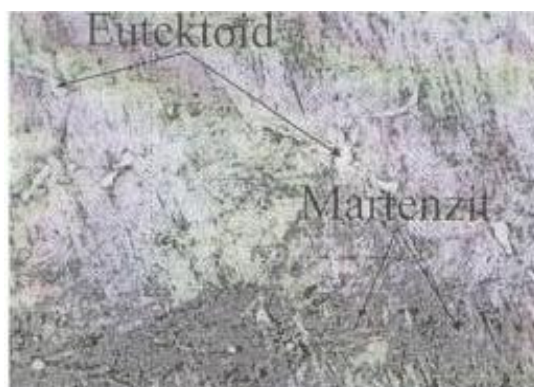
Figure 5 Microstructure of alloy quenched from 850°C and aged at 400°C for 1h (x960)
