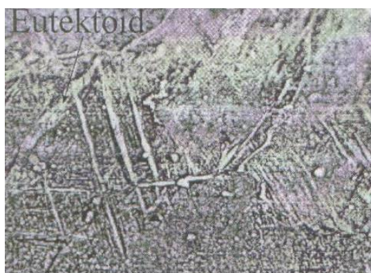
Figure 6 Microstructure of alloy quenched from 900°C and aged at 400°C for 1h (x960)
