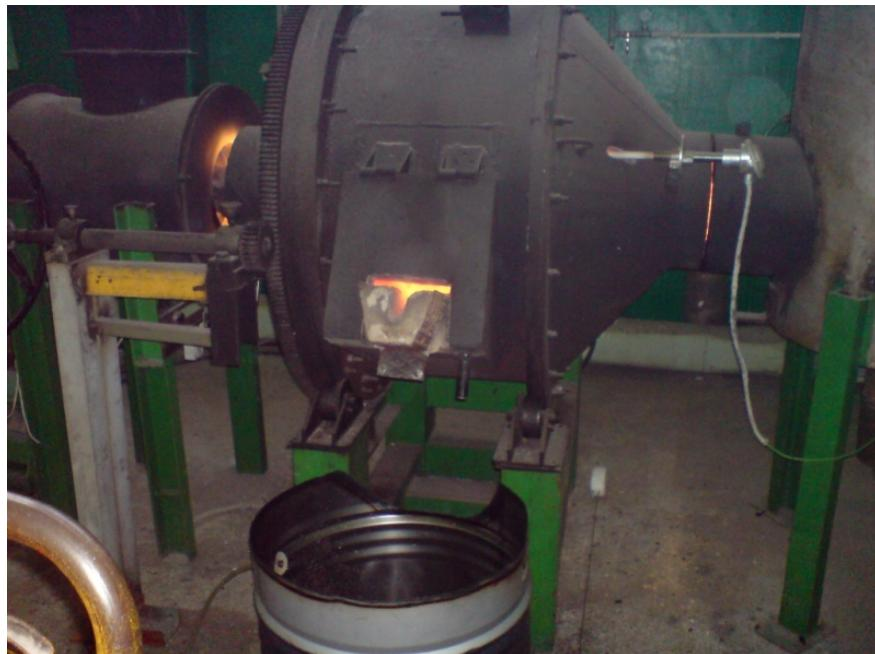
**Fig. 2.** Laboratory smelting furnace
