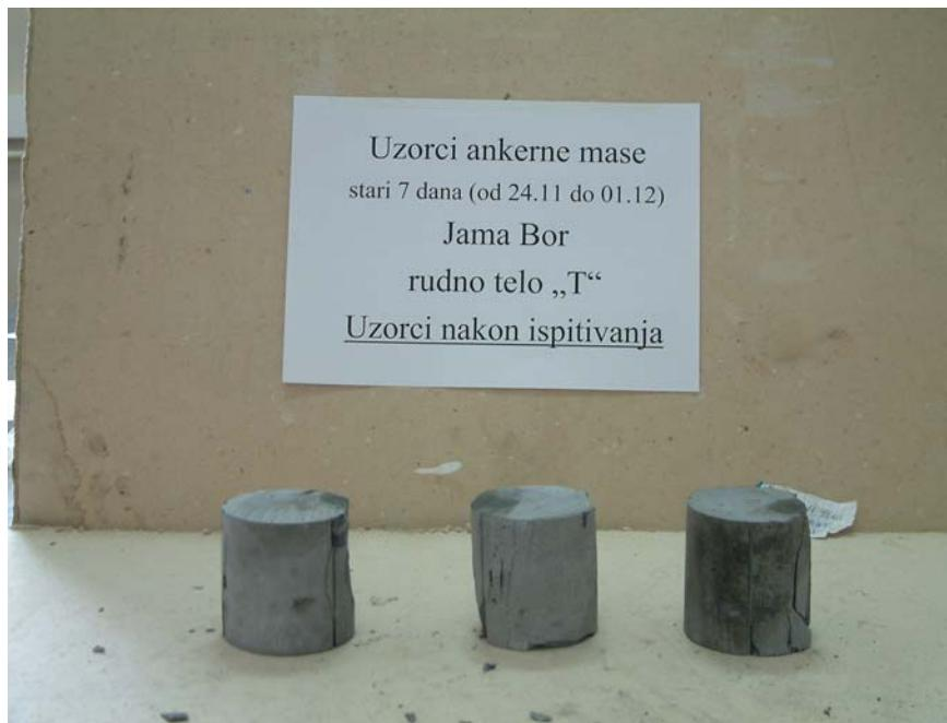
**Fig. 2.** Samples after testing
