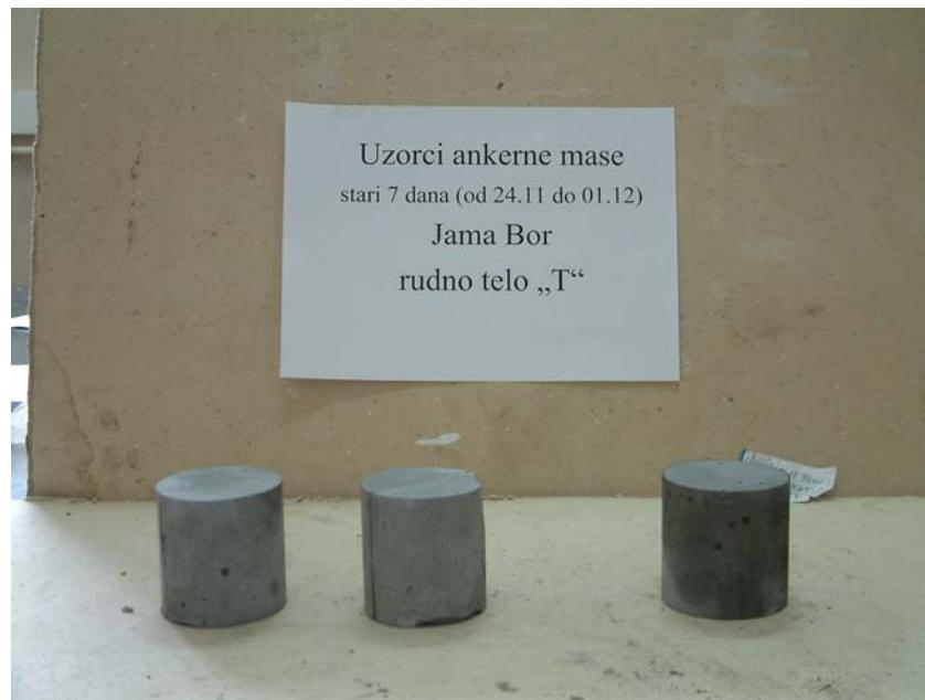
**Fig. 1.** Anchor mixture samples before testing
