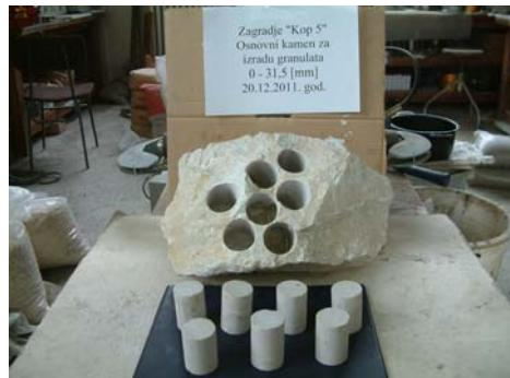
**Fig. 2.** Prepared samples for testing of a stone base
