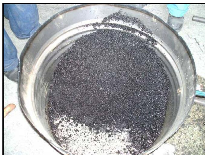
**Fig. 4.** The appearance of granulated slag
