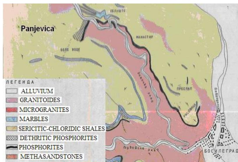
**Figure 1.** Geological map of the area of phosphorite sandstone deposit Lisina near Bosilegrad, Southeast Serbia
