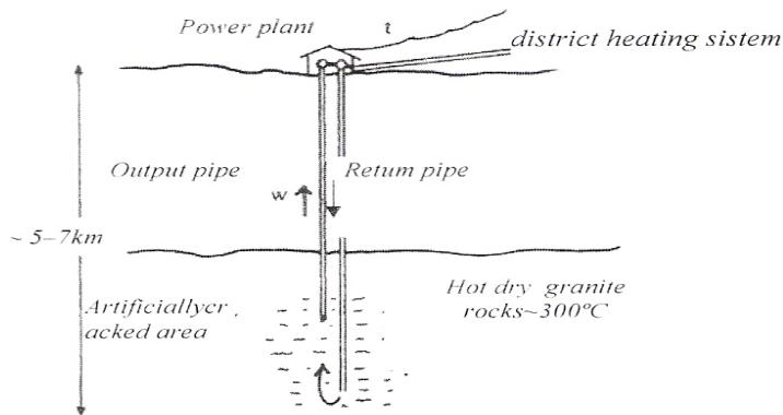
**Figure 1.** System for use the energy accumulated in dry rocks [1]
