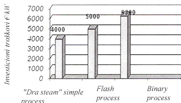
**Figure 5.** The investment cost of geothermal power plants, depending on the production process [4]
