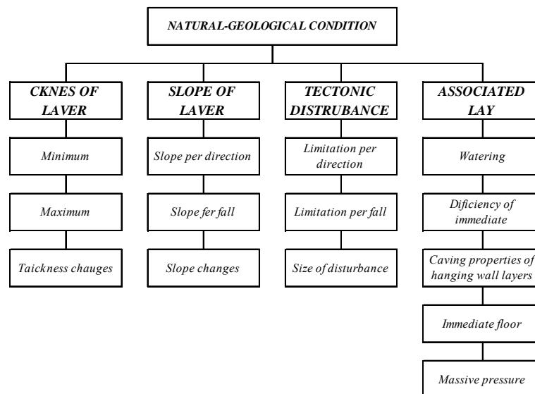
**Fig. 2.** Natural geological conditions in the selection of mining method with mechanized short face
