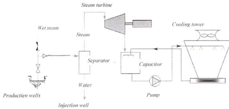
**Figure 3.** Schematic view of the flash conversion process the geothermal energy into electricity
