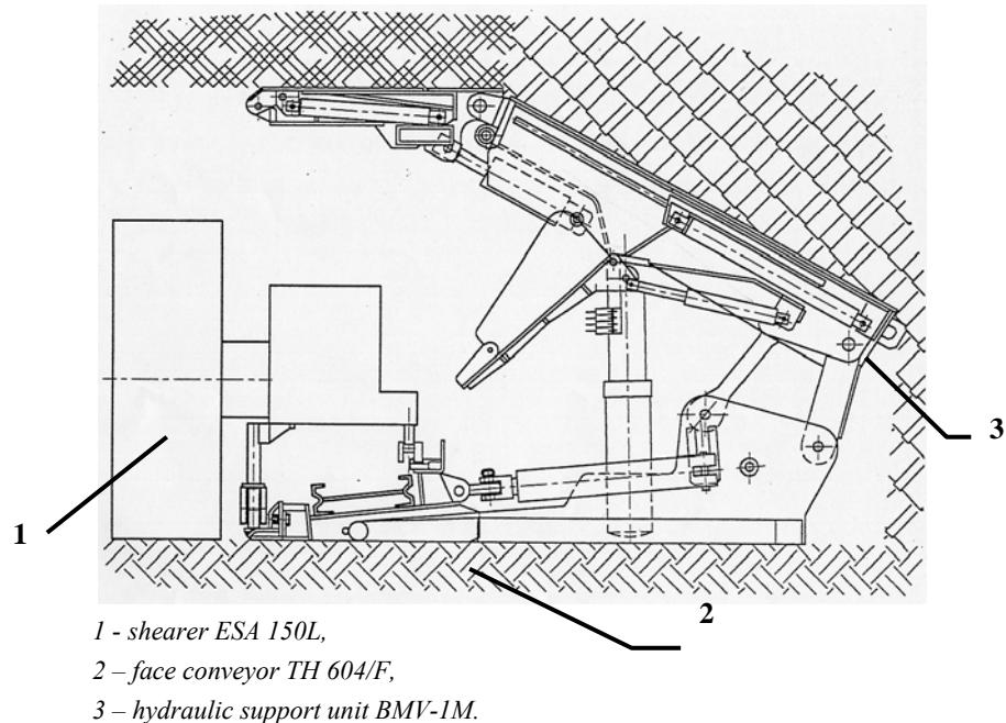
**Figure 1.** Schematic view of the mechanized long wall face
