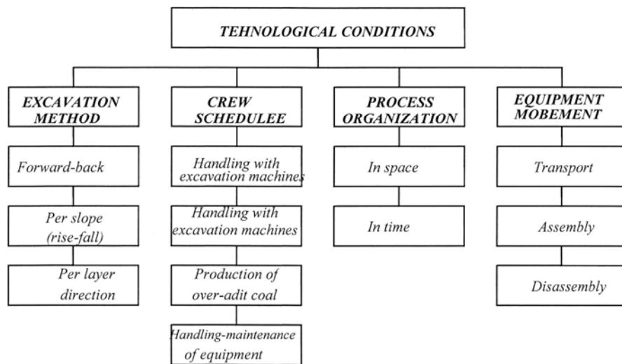
**Fig. 4.** Technological (organizational) conditions in the selection of mining method with mechanized short face with high concentration
