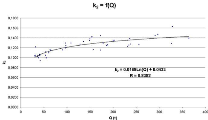
**Fig. 1.** Relationship between the coefficient  $k_2$  and the maximum truck payload  $Q$
