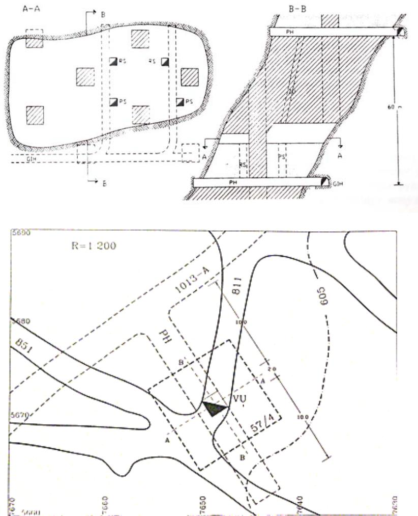
**Figure 1.** The Trepca mining method with the location of safety pillar
