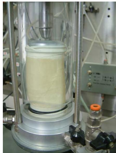
**Figure 2.** Sample after a failure stage
