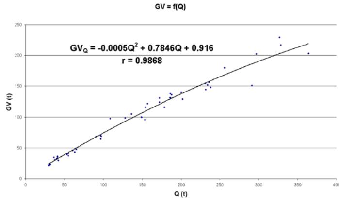
**Fig. 2:** Relationship between the truck weight  $GV$  and its maximum payload  $Q$
