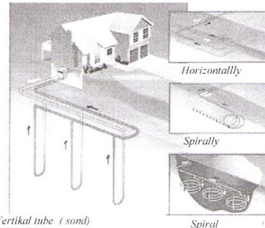
**Figure 6.** Heating systems with geothermal heat pumps (closed-circuit process)
