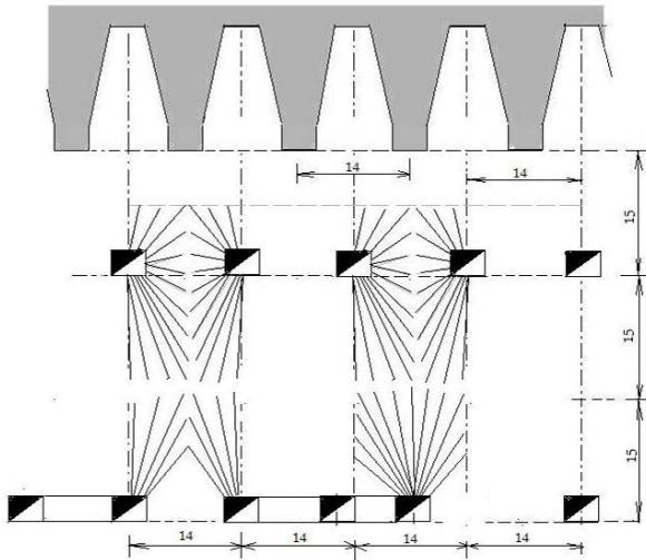
**Figure 6.** Proposal of the II variant of mining method with an open stope and sublevel drifts for drilling in the sides of mining block
