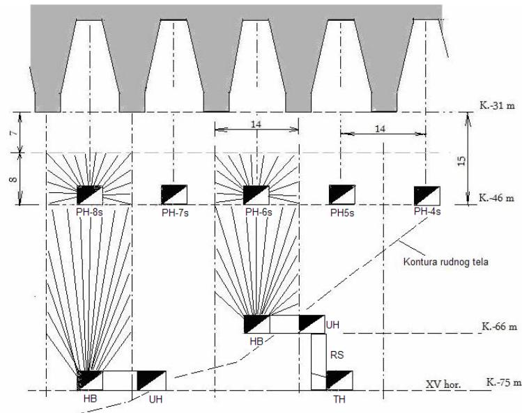
**Figure 5.** Proposal of the I variant of mining method with leaving the open slopes for excavation the lowest parts of the ore body Tilva Ros
