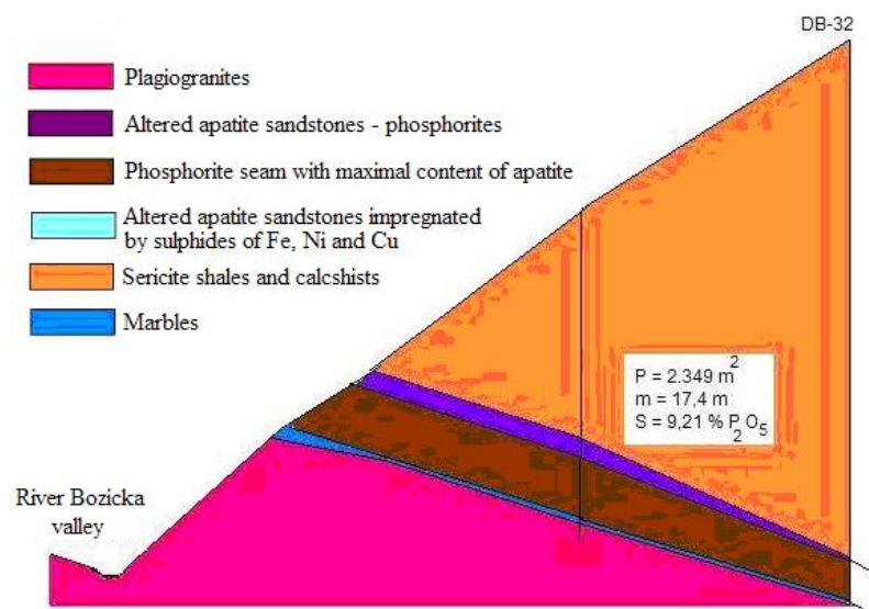
**Figure 2.** Vertical cross-section (No. 7) of the deposit
