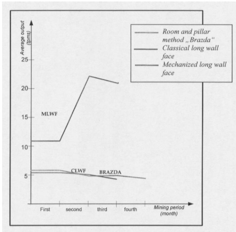
**Figure 2.** Diagram of output for excavation with different mining methods
