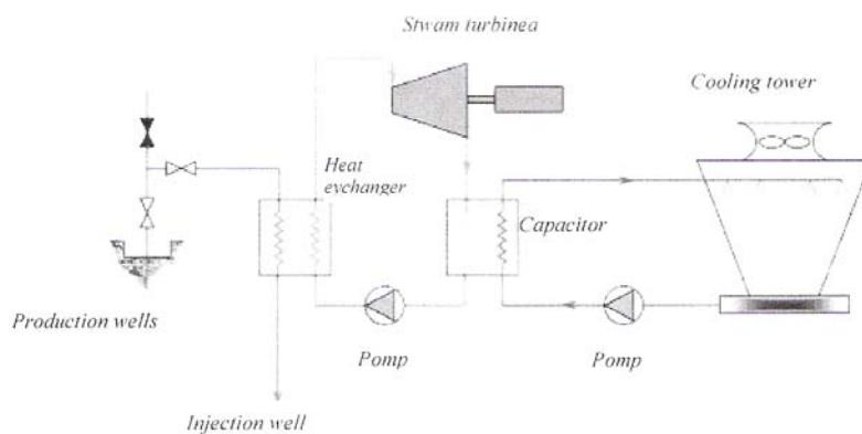
**Figure 4.** Schematic presentation of a binary geothermal conversion process into electricity
