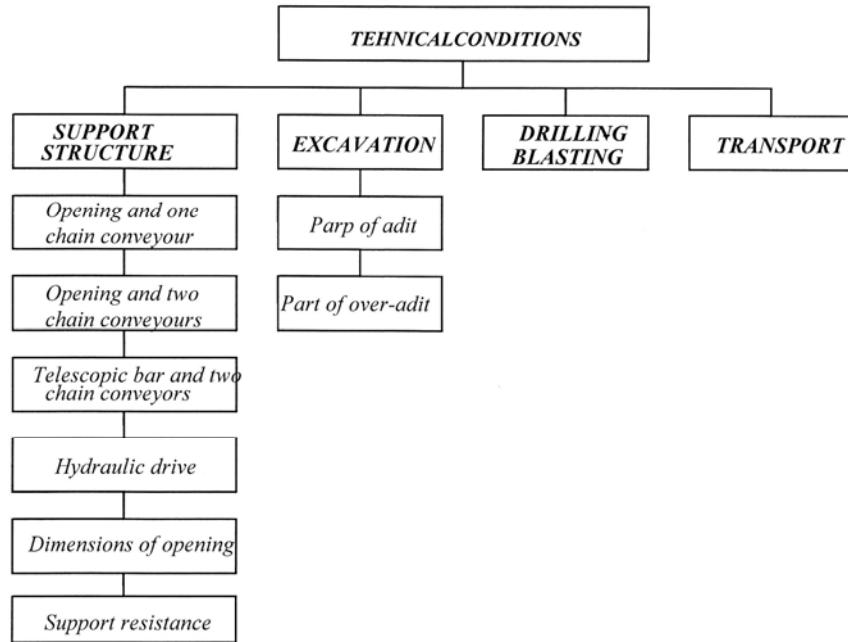
**Fig. 3.** Technical conditions in the selection of mining method with mechanized short face with high concentration
