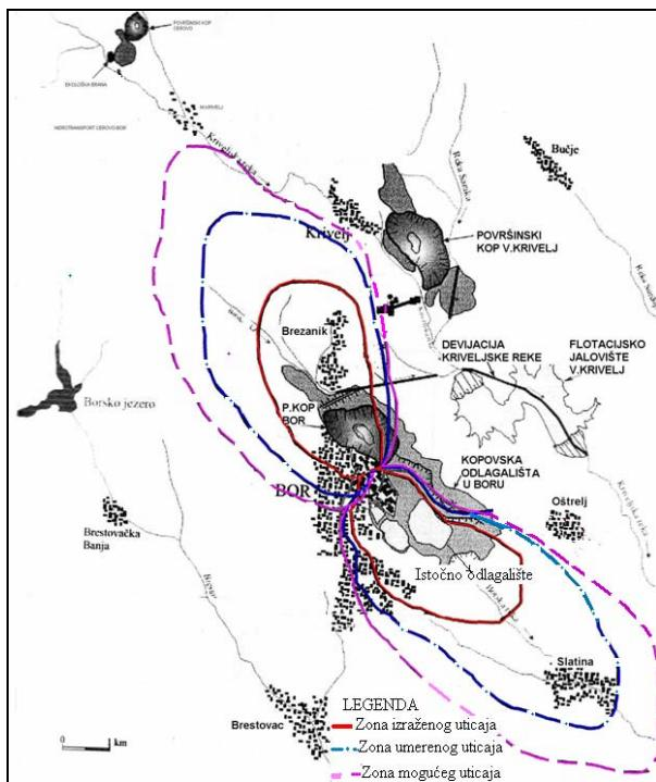
**Fig. 3. Zone of pollution influence from the Smelter stack in Bor**
