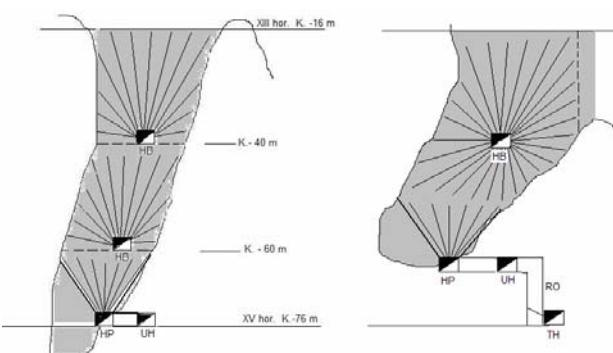
**Figure 8.** Proposed method of sublevel mining in the open stopes distributed per direction of the certain parts of the ore body
