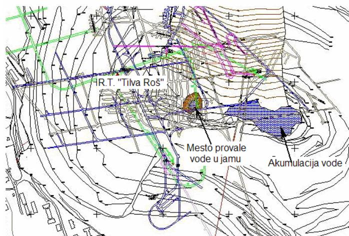
**Figure 1.** Situation in the open pit in Bor with the underground mining operations in the ore body Tilva Ros and marked place of water and mud influx in the pit
