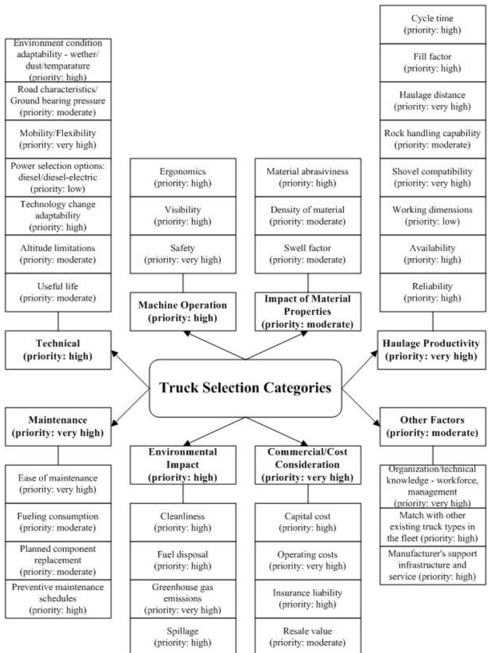
**Fig. 4.** A hierarchical structure of truck selection attributes and priority ranks
