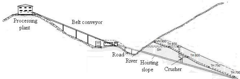
**Figure 5.** Proposed mine opening for the Lisina phosphorite deposit
