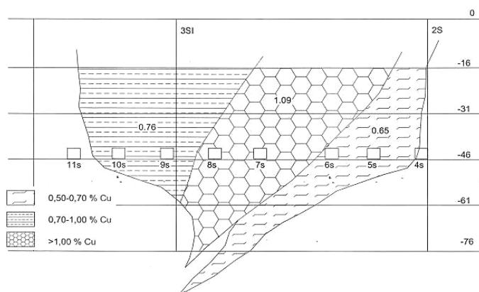
**Figure 3.** Longitudinal geological section 1 in the northern part of the ore body Tilva Ros
