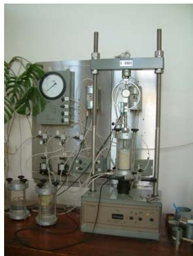
**Figure 1.** Triaxial apparatus
