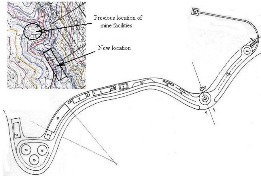
**Figure 6.** Layout of the mine facilities on the surface, the newly proposed location
