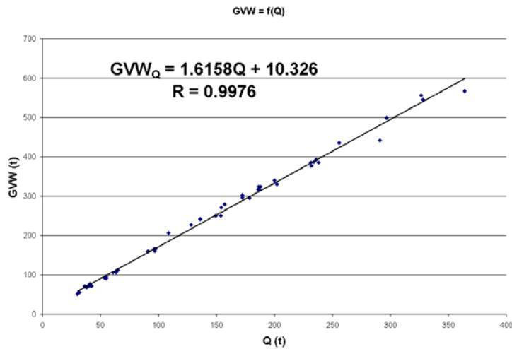
**Fig. 3:** Relationship between the gross truck weight  $GVW$  and its maximum payload  $Q$
