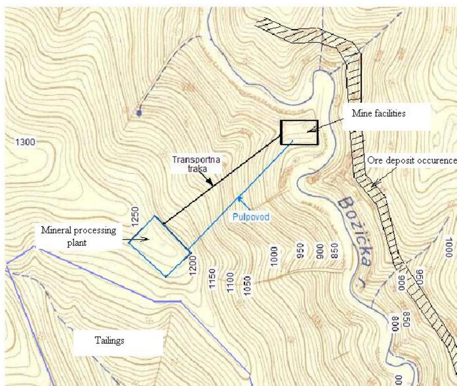
**Figure 4.** Layout of mine facilities, mineral processing plant and tailing dump by the first solution, proposed in 2008
