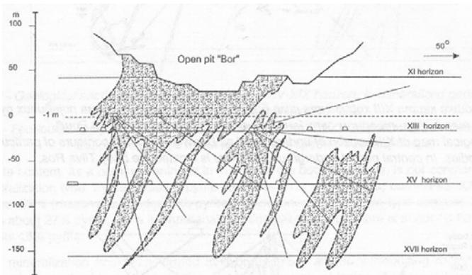
**Figure 7.** Cross section of lower part of the ore body Tilva Ros
