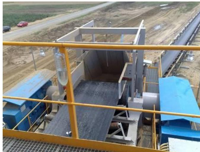
**Figure 2 Transfer chute and two gears connected with drive drum**
