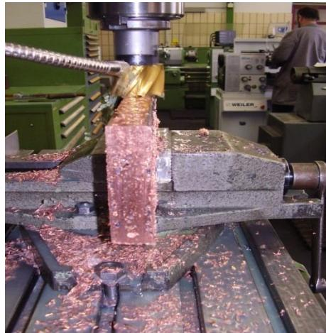
**Figure 1** Copper anode mechanical finishing
