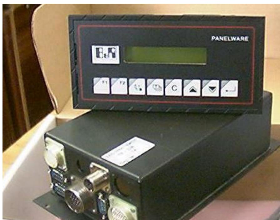
Figure 1 Load module with the panel
