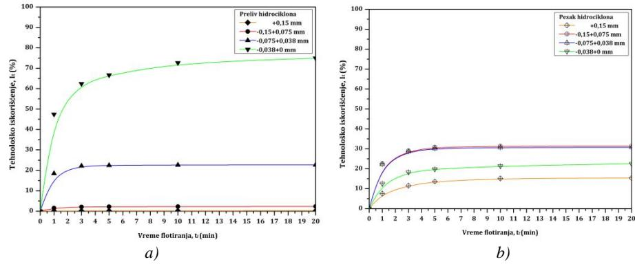
**Figure 4** Copper recovery by narrow size classes of classification products
