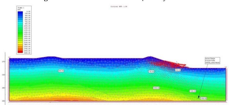
**Figure 4** The main normal stress  $\sigma_1$  in the second situation
