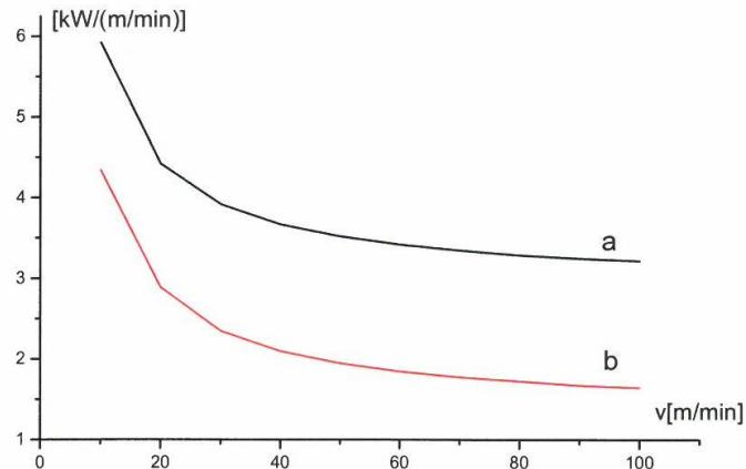
**Figure 8** Heat coefficient in the function of the production speed
