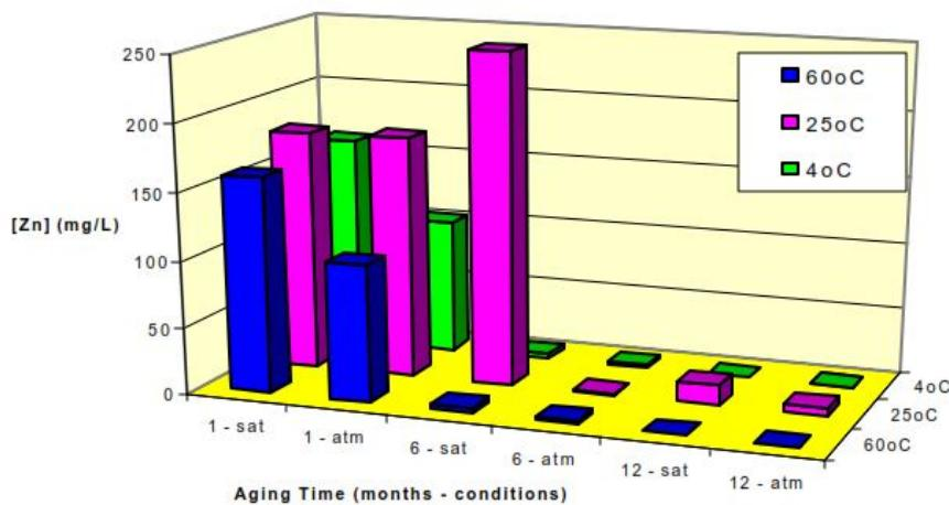
**Figure 3** Relationship between metal mobility and sludge aging
