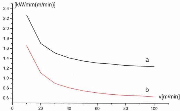
**Figure 9** Specific power in the function of the production speed
