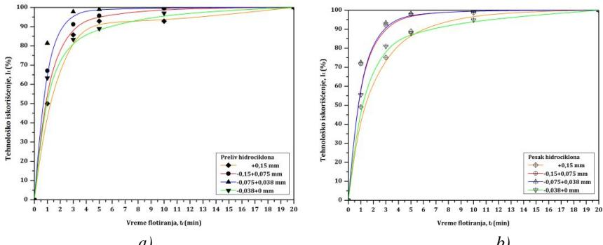
**Figure 3** Copper flotation kinetics from narrow size classes
