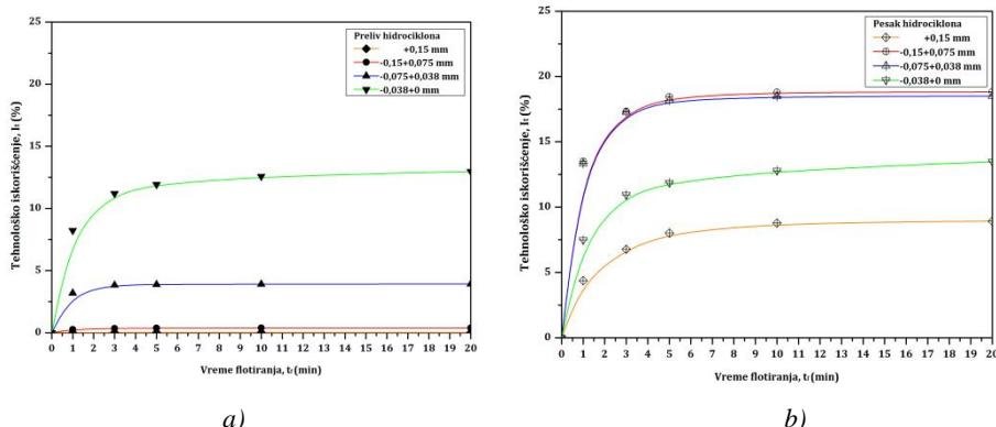
**Figure 5** Copper recovery by size classes, compared to the copper content in feed of hydrocyclone: a) hydrocyclone overflow b) hydrocyclone underflow
