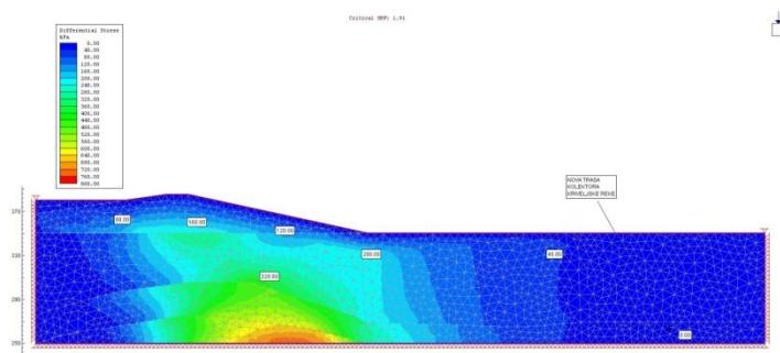
**Figure 7** Differential stress  $\sigma_{1-3}$  in the I situation
