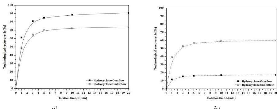
Figure 2 Copper flotation kinetics from hydrocyclone overflow and underflow
