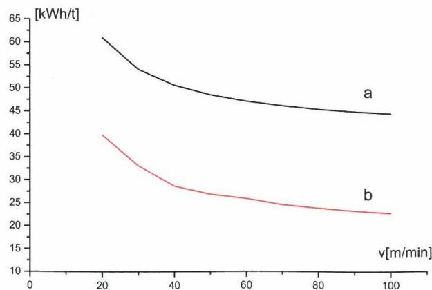
**Figure 7** Energy consumption as per tone of tube in the function of production rate
