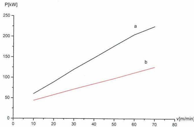
**Figure 5** Power from rectifier in the function of production rate
