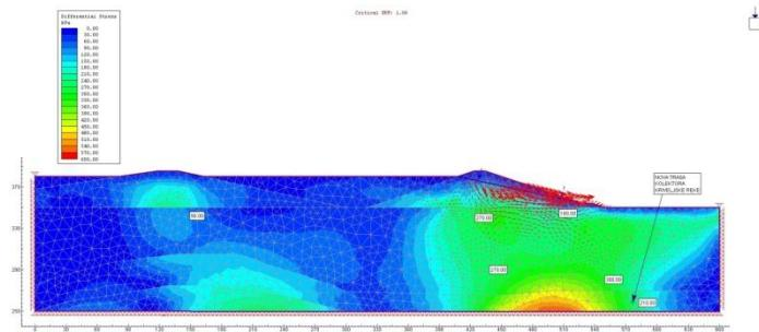
**Figure 8** Differential stress  $\sigma_{1-3}$  in the II situation
