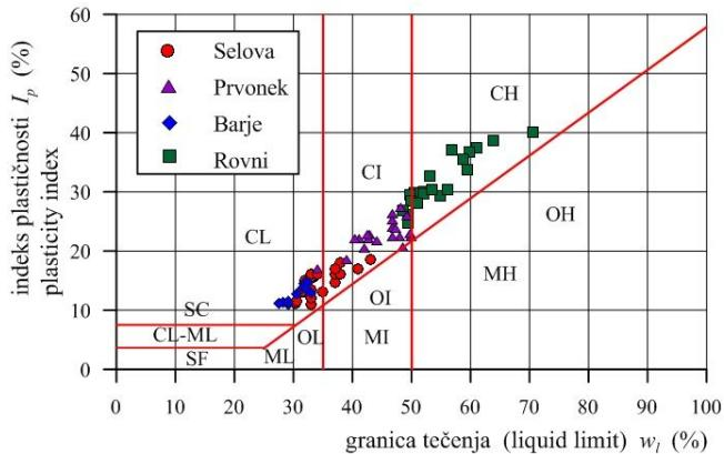
**Figure 2** Diagram of plasticity the tested clayey material
