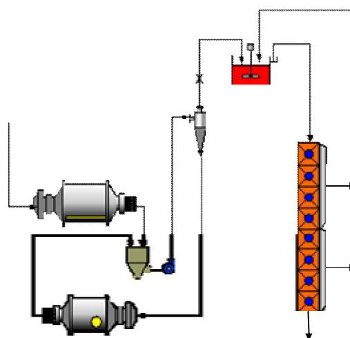
**Figure 1** Flowsheet of grinding and classification process of high-grade copper ore
