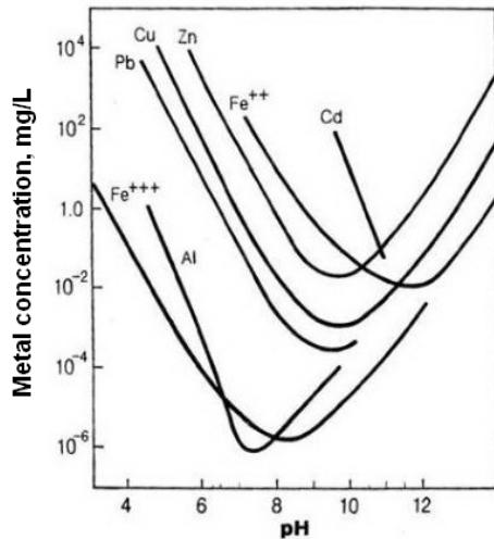
**Figure 2** Metal hydrolysis solubility curve
