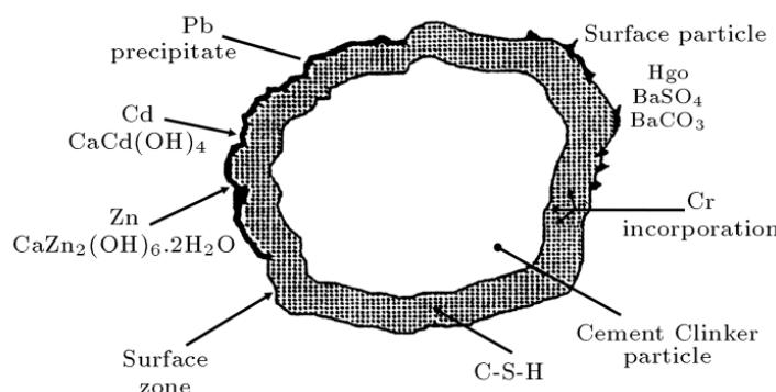
**Figure 1** Solidification and stabilization of heavy metals by hydrates of Portland cement [6]
