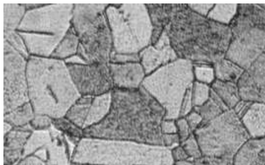
Figure 2. CuZnSnSiMn alloy after plastic deformation and heat treatment (magnification 400x)
