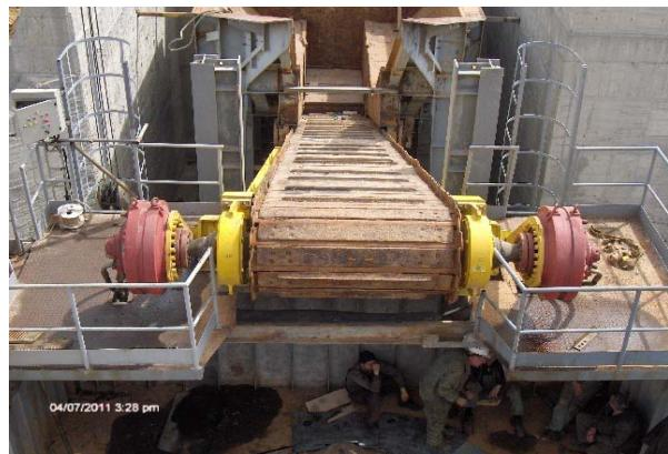
**Fig. 3.** Hydrodrive of the apron feeder
