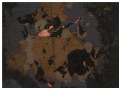
**Fig. 2. Intergrowth of chalcopyrite, pyrite and copper matte with separation of elemental copper, lens 50X, II Nikoli**
