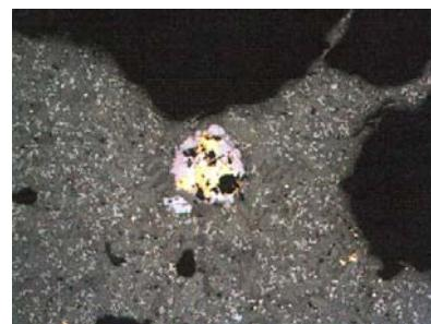
**Fig. 3. Intergrowth of chalcopyrite, pyrite and bornite in fayalitic basis, lens 10X, II Nikoli**
