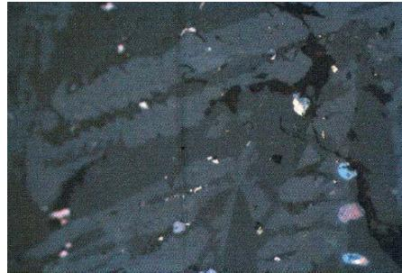
**Fig. 4.** Intergrowth of pyrite, chalcocite and copper matte, lens 50X, II Nikoli
