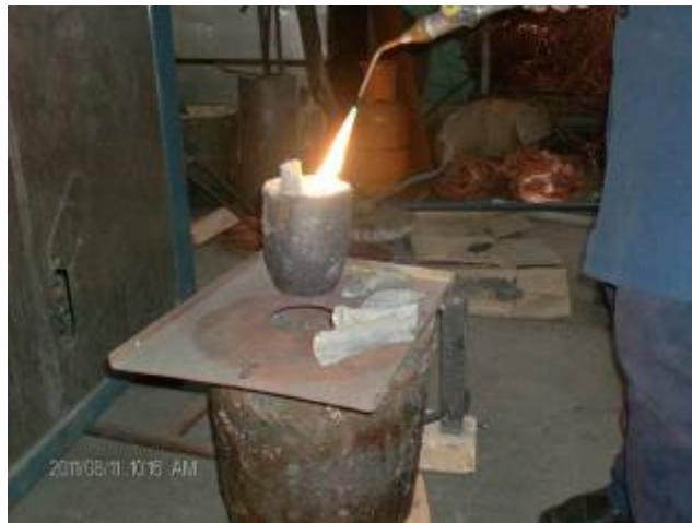
Figure 3. Graphite pot with autogenous smelting
