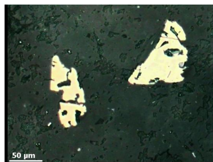
Figure 2 Aggregates of chalcopyrite (yellow) embedded in silicate substrate (dark-gray). Air, II N.
