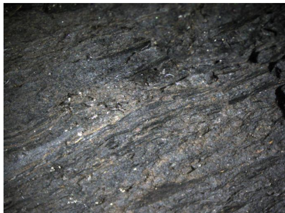
Figure 3 Xylite, binocular, magnification 6.5 x
