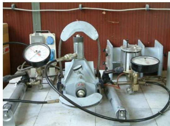
**Fig. 4.** Apparatus for shearing
