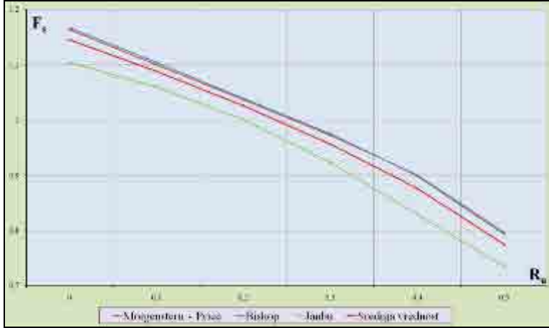
Figure 8. Graph of the stability coefficient F_s depending on the pore water R_u
