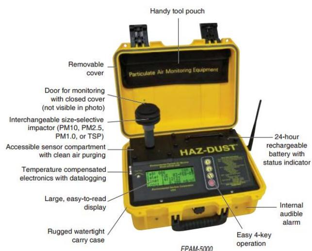
**Figure 2** Front panel of the EPAM-5000 monitor
