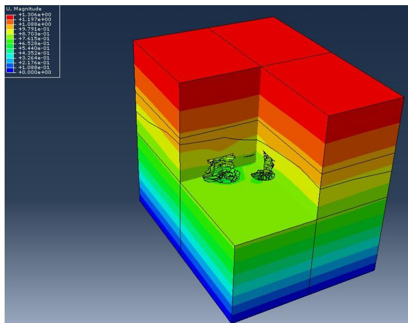
**Figure 4** Magnitude of displacements in cavern cross section
