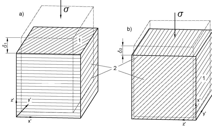
**Figure 3 Deformation anisotropy of rocks with a layered structure**
