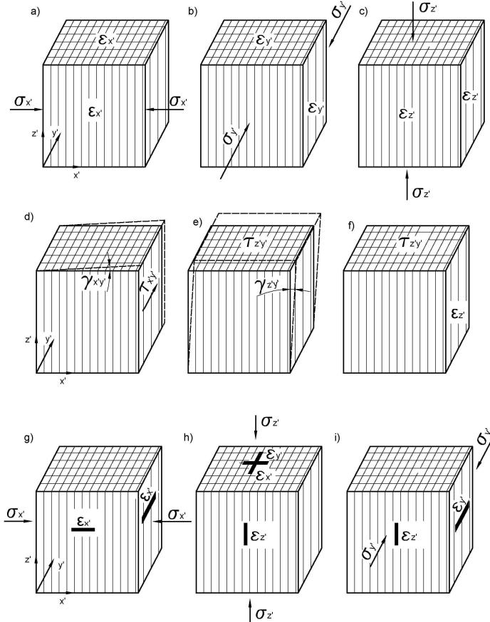
**Figure 4** Determination the elastic constants for rocks in the case of transverse complexion for isotropic layered structure
