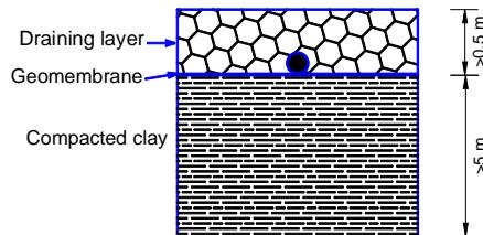
**Figure 2** Detail "A" - Sealing/drainage structure of bottom and slopes
