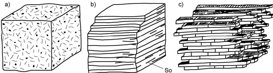
**Figure 1 Structural rock model**
