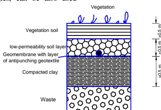
**Figure 3** Detail "B" - Design of coverage layer
