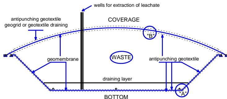
**Figure 1** A typical cross section of the hazardous waste landfill
