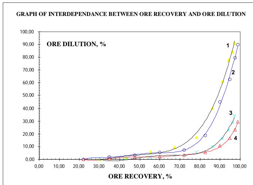
**Figure 4** Relation between the ore recovery and ore dilution in case of ore drawing from two and three draw points, with optimal values of method parameters
