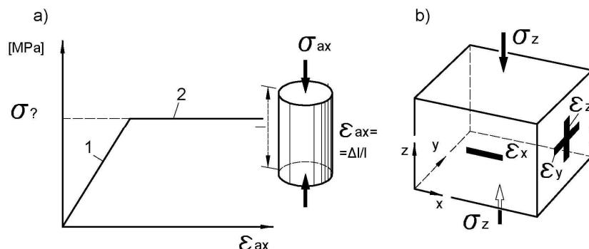
**Figure 2 Deformability of isotropic rocks**
