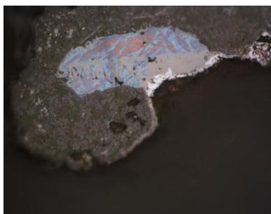
**Figure 3** Copper matte, bornite and chalcopyrite, magnification 500 x II N
