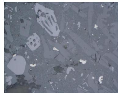
**Figure 8** Magnetite in various forms, magnification 500 x II N
