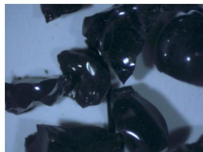
**Figure 2** Grains of granulated slag (sharp edges), binocular, magnification 2.0 x
